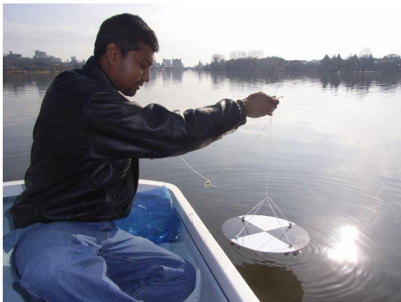
Fig.4. Measuring water transparency using Secchi disk at Senba Lake, Japan during our previous studies.
