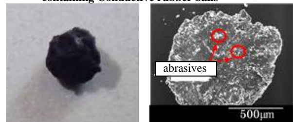
Fig.2 Developed conductive rubber ball and surface composition
